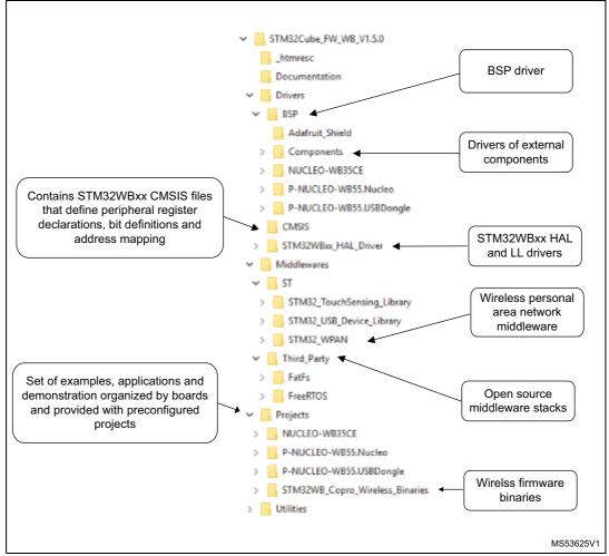
Figure 3. STM32CubeWB firmware package structure
