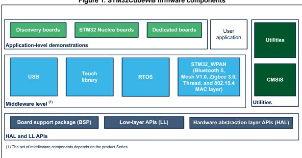
Figure 1. STM32CubeWB firmware components
