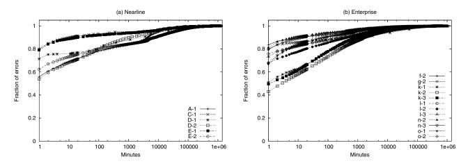
Figure 7: Inter-arrival rate. The graphs show the cumulative distribution of the inter-arrival rates of latent sector errors per minute. The fraction of errors per model is plotted against time. The arrival rates are binned by minute.
