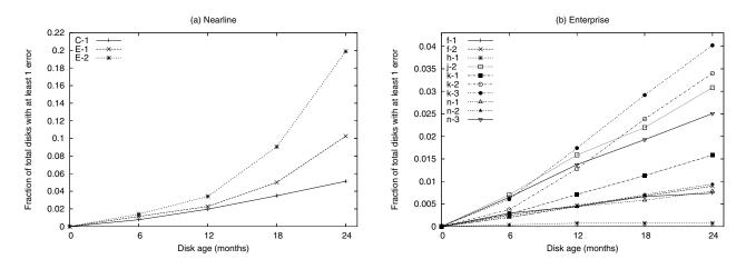
Figure 1: Impact of disk age. The probability that a disk develops latent sector errors as it ages is shown. Note that the probability is cumulative. Also, note that the y-axis scale is different for the two graphs.
