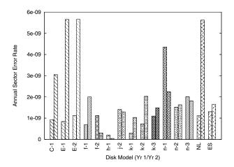
Figure 2: Annual sector error rates (ASERs). For each disk model that has been in the field for at least two years, the first bar represents Year 1 and the second represents Year 2. The NL and ES bars represent weighted averages for nearline and enterprise class drives respectively.
