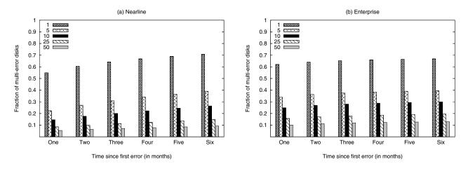
Figure 8: Temporal decay. The probability of experiencing at least 1, 5, 10, 25, and 50 additional latent sector errors within a given time period since the occurrence of the first error.
